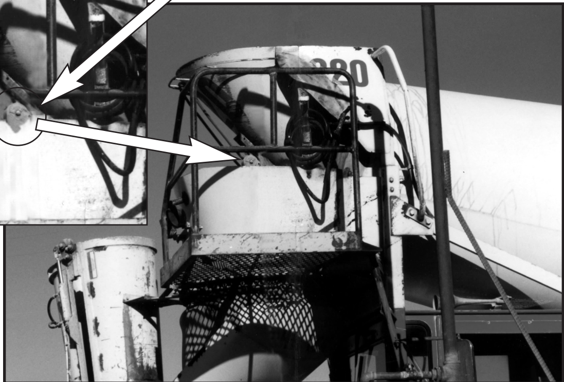
A VS-250 Air Turbine Vibrator mounted on a charge hopper of a front discharge mixer truck.
