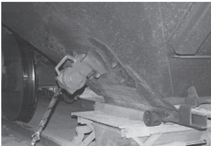
SVRWS-6500 Unloading Silica Sand
